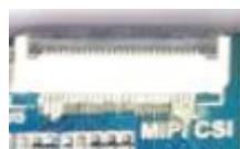
This interface is the common 26PIN camera interface, support OV, Himax camera, save the camera switch board. In view of the different types of cameras, only in accordance with the camera specification, adjust the output voltage on the line.
