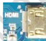
G4418 development board uses miniHDMI interface, with the miniHDMI extension cable, audio and video signal can be the perfect present in the monitoring terminal, to support the HDMI1.4 protocol as a TV set, display etc.
