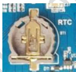
The backup battery is used to ensure that the RTC is still able to work after power failure and the system time is not lost. When G4418 development connects a lithium battery, it will supply power to the RTC, RTC will not be lost if the battery isn't off, so G4418 development board won't provide RTC backup battery.
