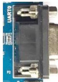
G4418 development board reserves a RS232 serial port UART0, as the default debug serial port. And there are 2 TTL serial port, UART1 , UART2.
