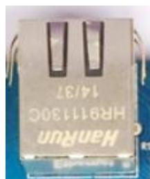
G4418 development board supports Gigabit wired Ethernet interface, collect RTL8211E onboard, users can access through a wired Ethernet.
