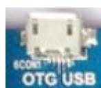
This interface is used to write the program, synchronization. It can use as HOST with OTG cable.
