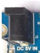
G4418 development board takes 5V DC power supply, and the black jack in the picture is 5V DC power input jack.
