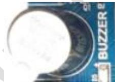
The buzzer is active buzzer will sound when DC passes, the power on or off is controlled by the transistor. The transistor is controlled by one channel PWM, can use for testing PWM or voice prompt in suitable situation.
