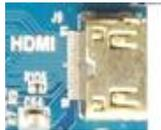
G6818 development board uses mini HDMI interface, with the mini HDMI extension cable, audio and video signal can be the perfect present in the monitoring terminal, to support the HDMI1.4 protocol as a TV set, display etc.
