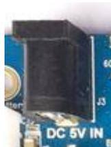
G6818 uses 5V/2A DC power supply, and the black jack in the picture is 5V DC power input jack.
