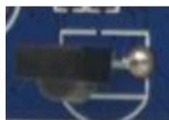
Here we used HS0038B integrated receiver, it has the high sensitivity and easy to use. We can realize the wireless remote control and make the G6818 development board as a
