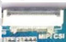
This interface is the common 26PIN camera interface, supportS OV, Himax camera, save the camera switch board. Users just need to adjust the output voltage according to the specifications of the camera for different types of cameras.
