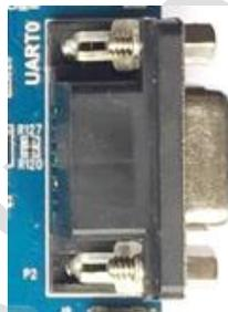
G6818 reserve a RS232 serial port UART0, as the default debug serial port. UART1 is RS232, UART2 is TTL.
